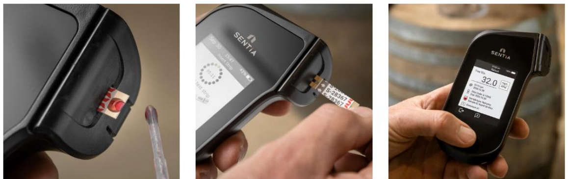
Above: Sentia Wine Analyser electrochemical test strips and portable meter (reader device).
