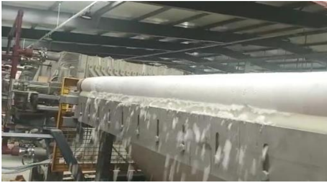
Figure 1: First lithium coming off the vacuum filter at the 2ktpa facility. The company expects production and product quality to ramp up over the coming months
